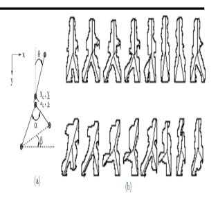
Figure 4: (a) Determining of posture features from the skeleton, (b) Silhouette and skeleton motion sequences of a walking and running person, respectively.
